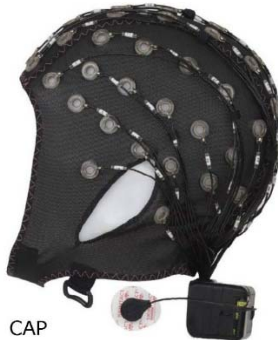
Figure 9: Cognionics Mobile Series Headset EEG Cap and Harness
